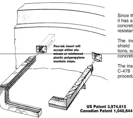
Since the insert is made of polypropylene, it has a life expectancy which exceeds the concrete itself, and has excellent chemical resistance.
